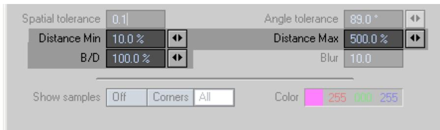
**Distance Min/Max** : this controls minimum and maximum distance between samples. If min and max are exactly the same, samples will be distributed equally apart across all surfaces (and we don't want that).
